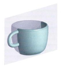
Three-dimensional objects with reflectional symmetry can be divided into two congruent parts by a plane. You can sketch these symmetries in two dimensions by using orthographic views (top, front, or right side).
