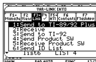
An analogous procedure can be used to send applications between calculators. Applications (such as the Statistics with List Editor) are selected from the [F7]FlashApp menu (press [2nd][F2] for [F7].)
