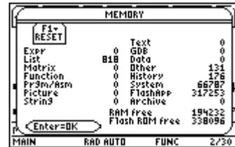
To delete lists which are no longer needed, press **2nd**- (VAR-LINK). Move the cursor to highlight the list to be deleted, then press **F1**. Press **ENTER** to select option 1:Delete.
