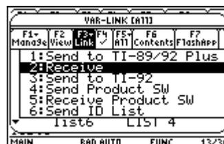
On the sending calculator, use the arrow keys to select the item to send, then press [F4] to “check” the item. The example at right will send list1 and list2.
